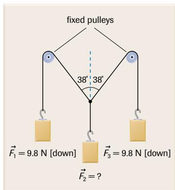
The above diagram shows a possible setup for a vertical force board. (You may prefer to modify the setup, however, using a force table instead of a force board, as suggested for this activity.) In this vertical force board, there are three different forces, each acting on a different string. If two of the forces are known, the third force can be determined. Describe how you would determine the unknown force  $\vec{F}_2$ .
