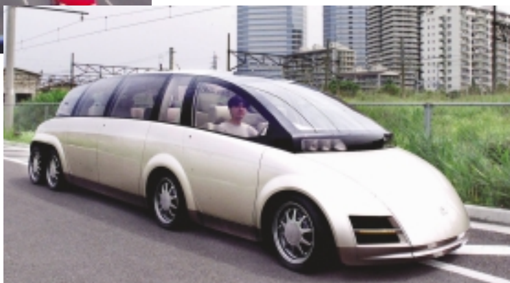
Figure 2 This experimental electric limousine, with a mass of 3.0 \times 10^3 kg, can travel 300 km on an hour's charge of its lithium battery.
