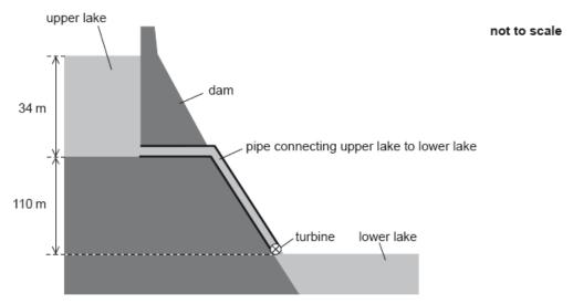
The water leaving the upper lake descends a vertical distance of 110 m and turns the turbine of a generator before exiting into the lower lake.
