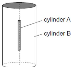
At the start of the experiment all the air was removed from cylinder B. The alpha particles combined with electrons as they moved through the wall of cylinder A to form helium gas in cylinder B.
