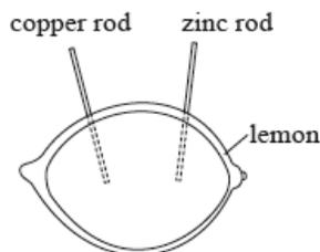
A student constructs a lemon cell and connects it in an electrical circuit with a variable resistor. The student measures the potential difference  $V$  across the lemon and the current  $I$  in the lemon.
