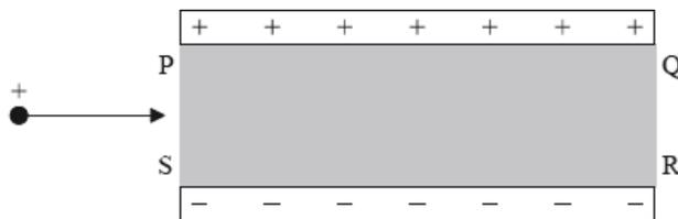
The top plate is positively charged and the bottom plate is negatively charged. There is a magnetic field in the shaded region PQRS. The particle continues to move in a horizontal straight line between the plates. Which of the following correctly describes the magnetic field direction?
