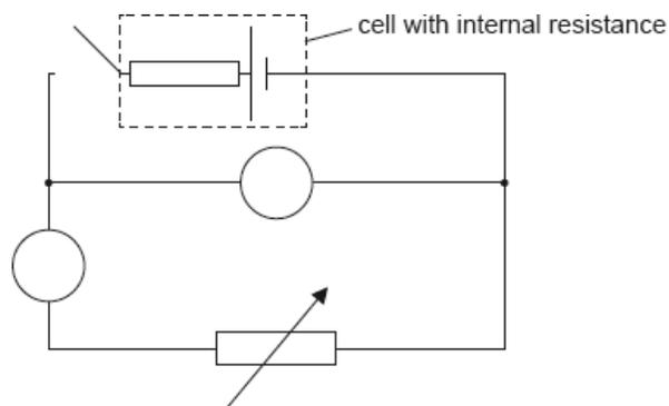
14a. An ammeter and a voltmeter are connected in the circuit. Label the ammeter with the letter A and the voltmeter with the letter V.
