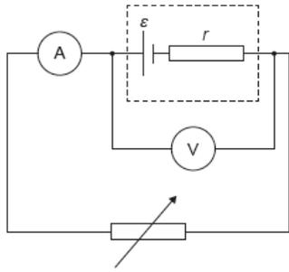
The current  $I$  and the terminal potential difference  $V$  are measured.
