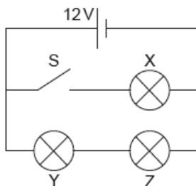
2a. The switch S is initially open. Calculate the total power dissipated in the circuit. [2 marks]
