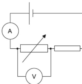
What changes occur in the ammeter reading and in the voltmeter reading when the resistance of the variable resistor is increased?
