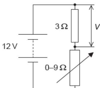
The power supply has an emf of 12 V and negligible internal resistance. What is the difference between the maximum and minimum values of voltage  $V$  across the 3  $\Omega$  resistor?
