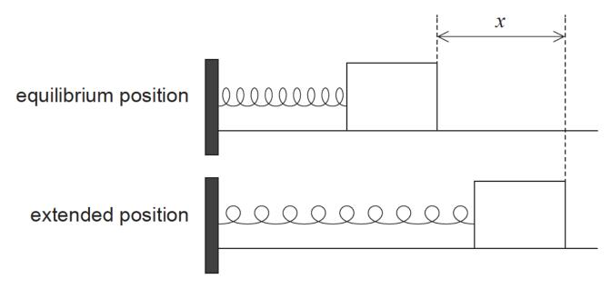
The tension F in the spring is given by F = k x where x is the extension of the spring and k is a constant.
