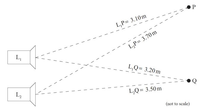
The waves leaving  $L_1$  and  $L_2$  are in phase and are observed at points P and Q.
