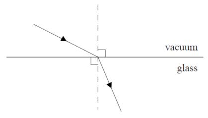
In glass, light has speed  $\nu$ . In a vacuum, light has speed c. Which of the following gives the refractive index of glass?
