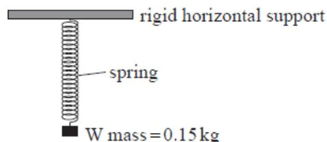
An object  $W$  of mass  $0.15 \text{ kg}$  is suspended from the other end of the spring. The extension  $x$  of the spring is proportional to the force  $F$  causing the extension. The force per unit extension of the spring  $k$  is  $18 \text{ Nm}^{-1}$ .
