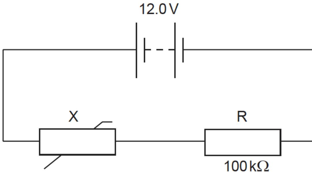
The battery has an electromotive force (emf) of  $12.0\text{ V}$  and negligible internal resistance.
