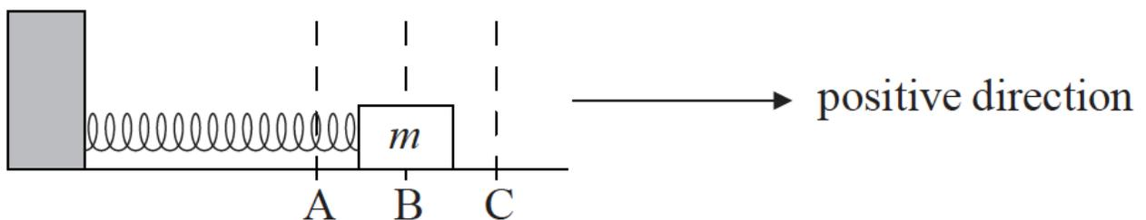
The equilibrium position is at B. The direction B to C is taken to be positive. The object is released from position A and executes simple harmonic motion between positions A and C.
