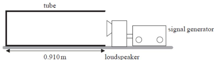
The frequency of the sound is slowly increased from zero. At a frequency of 92.0 Hz the first large increase in the intensity of the sound is heard.
