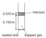
When the mercury is above the gas column the length of the gas column is 0.190 m.
