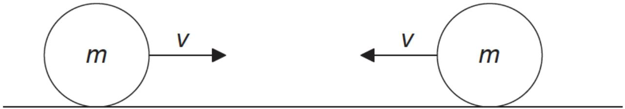
The spheres undergo a head-on elastic collision.
