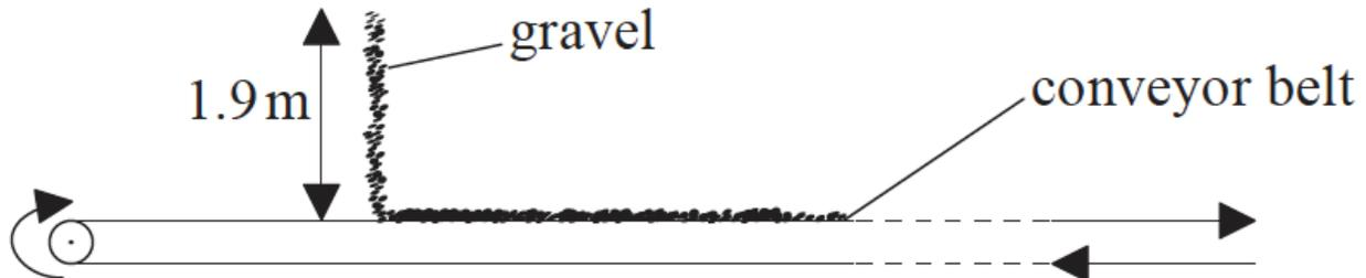
(i) The gravel falls at a constant rate of  $13 \text{ kg s}^{-1}$  through a height of  $1.9 \text{ m}$ . Show that the vertical speed of the gravel as it lands on the conveyor belt is about  $6 \text{ m s}^{-1}$ .
