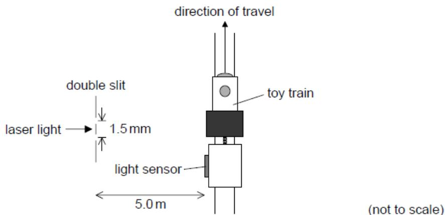
Light from a laser is incident on a double slit. The light from the slits is detected by a light sensor attached to the train.
