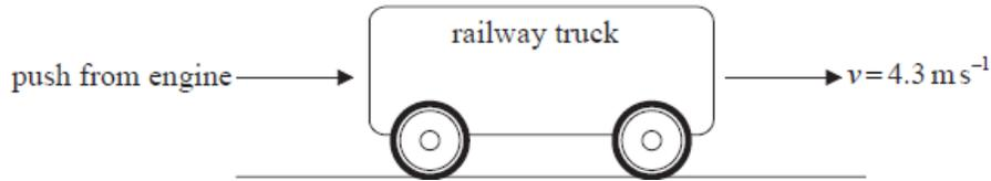
The engine is in contact with the truck for a time  $T = 0.54$  s and the initial speed of the truck after the push is  $4.3 \text{ ms}^{-1}$ . The mass of the truck is  $2.2 \times 10^3$  kg.
