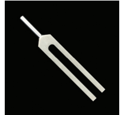
Figure 2 Tuning forks are available in different frequencies. A light tap to one tine (prong) of the fork sets both tines vibrating at a particular frequency.
