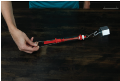
Figure 2 A force sensor is used to pull an object horizontally. Static friction keeps the object at rest.
