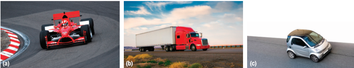
Figure 1 (a) A race car speeds up quickly because it has a small mass and experiences a large net force. (b) A truck accelerates more slowly. Even though a large net force acts on it, the mass is large. (c) A small economy car also accelerates more slowly. It has a small mass and a small applied force.
