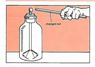
An electroscope is a simple instrument. It tells us if an object has static electricity.
