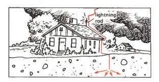
Every house should have a lightning rod. The lightning hits the lightning rod instead of the house.
